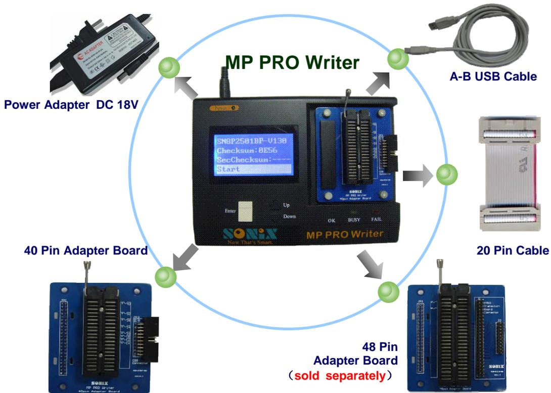
Figure 1-1 MP PRO Writer and accessories diagram
