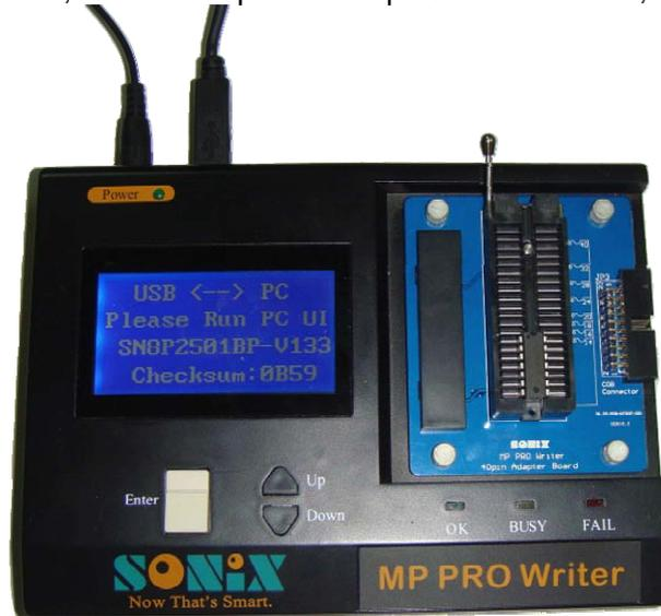
Figure 2-1 MP PRO Writer hardware connection
