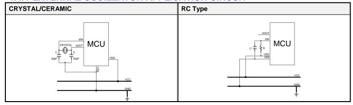
Note: Connect the Crystal/Ceramic and C as near as possible to the XIN/XOUT/VSS pins of micro-controller. Connect the R and C as near as possible to the VDD pin of micro-controller.
