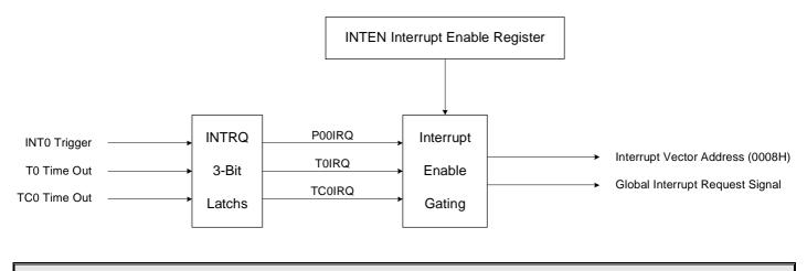
Note: The GIE bit must enable during all interrupt operation.
