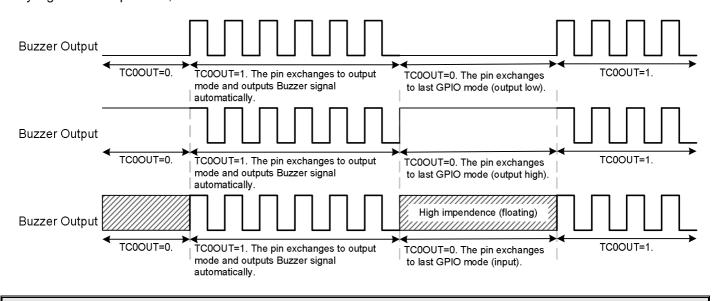
Note: Because the TC0OUT decides the PWM cycle in PWM mode. The PWM0OUT bit must be "0" when buzzer output function works.
