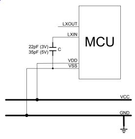
The external low clock supports watchdog clock source and system slow mode controlled by CLKMD.
