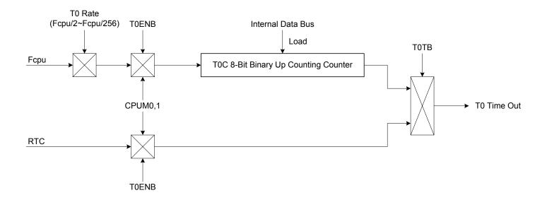
Note: In RTC mode, the T0 interval time is fixed at 0.5 sec and isn't controlled by T0C.
