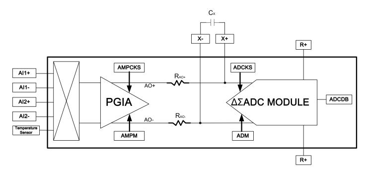
**Block Diagram of PGIA/ADC module**
