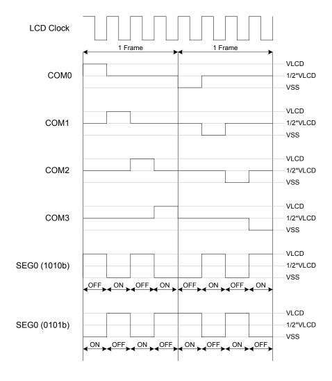
LCD Drive Waveform, 1/4 duty, 1/2 bias
