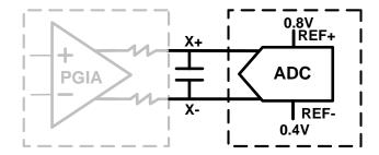
ADCM=#xxx0111xB, V(REF+, REF-) = V(1.2V, 0.4V)=0.8V (AVE+=3.0V), ADC Reference Voltage from Internal 1.2V and 0.4V, and ADC output is Voltage measurement result.
