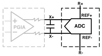
ADCM=#xxx0110xB, V(REF+, REF-) = V(1.2V, 0.4V)=0.8V (AVE+=3.0V) ADC Reference Voltage from Internal 1.2V and 0.4V.
