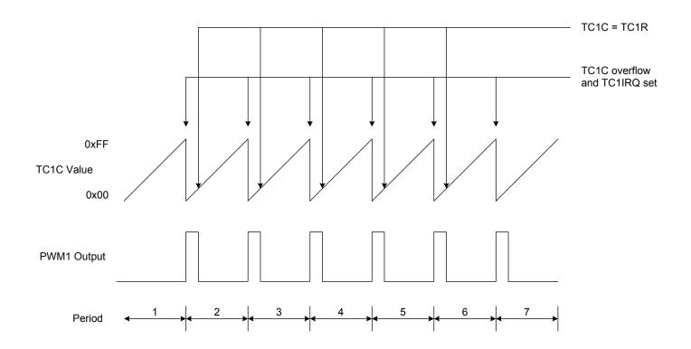
Above diagram is shown the waveform with fixed TC1R. In every TC1C overflow PWM output "High, when  $TC1C \ge TC1R$  PWM output "Low".
