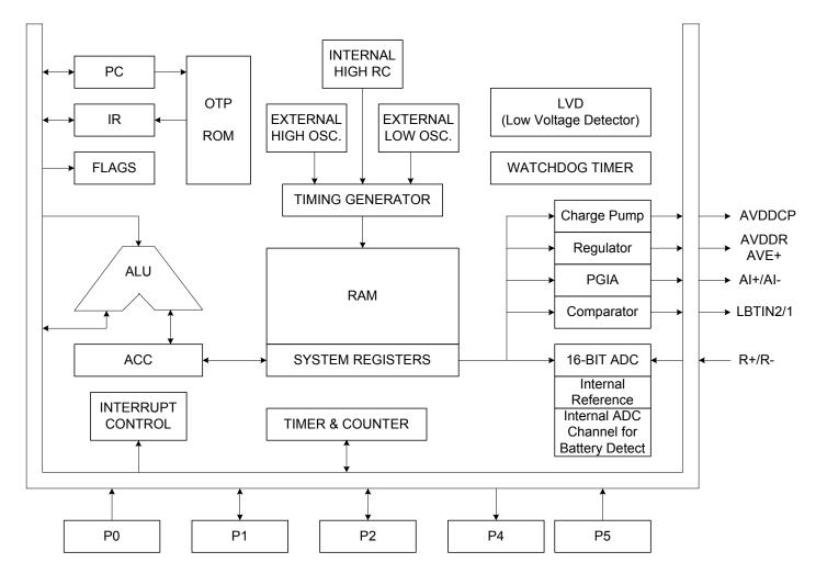
Figure 1-1 Simplified system block diagram
