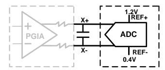
ADCM=#xxx0010xB, V(REF+, REF-) = V(0.8V, 0.4V)=0.4V (AVE+=3.0V), ADC Reference Voltage from Internal 0.8V and 0.4V.
