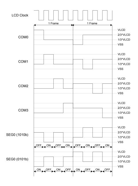
LCD Drive Waveform, 1/4 duty, 1/3 bias
